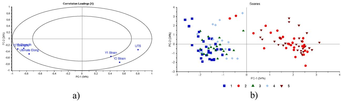
**Fig. 5.** PCA performed on the six characteristic points of each tensile curve for the EVA bags obtained for the 2 lots and all the gamma doses. a) Score plots with seal locations. b) Correlation loading (ellipses represent, from outside to inside, 75 % and 100 % of the correlation).
