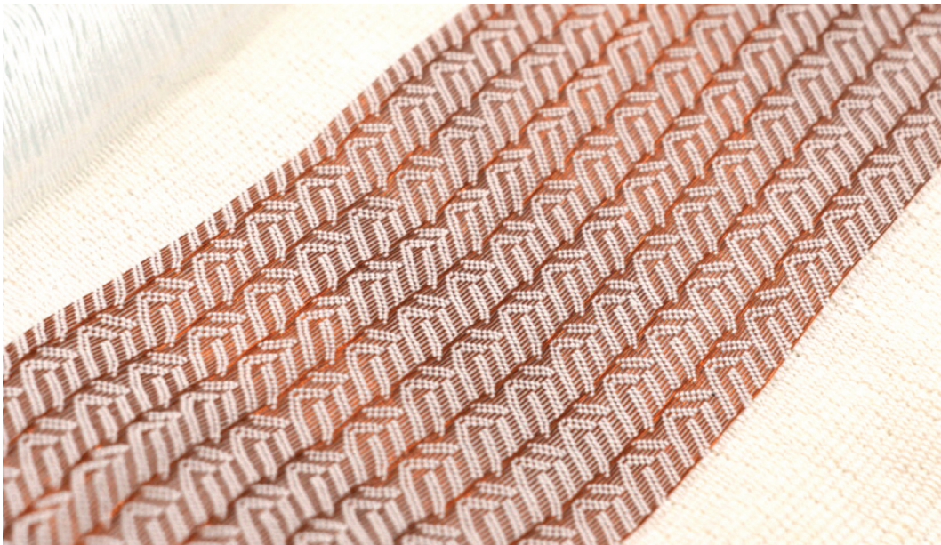
Figure 18: Diffusion of the electromagnetic field by increasing the amount of dielectric yarns that sit on the surface of the textile. © Erin Lewis (2021).
