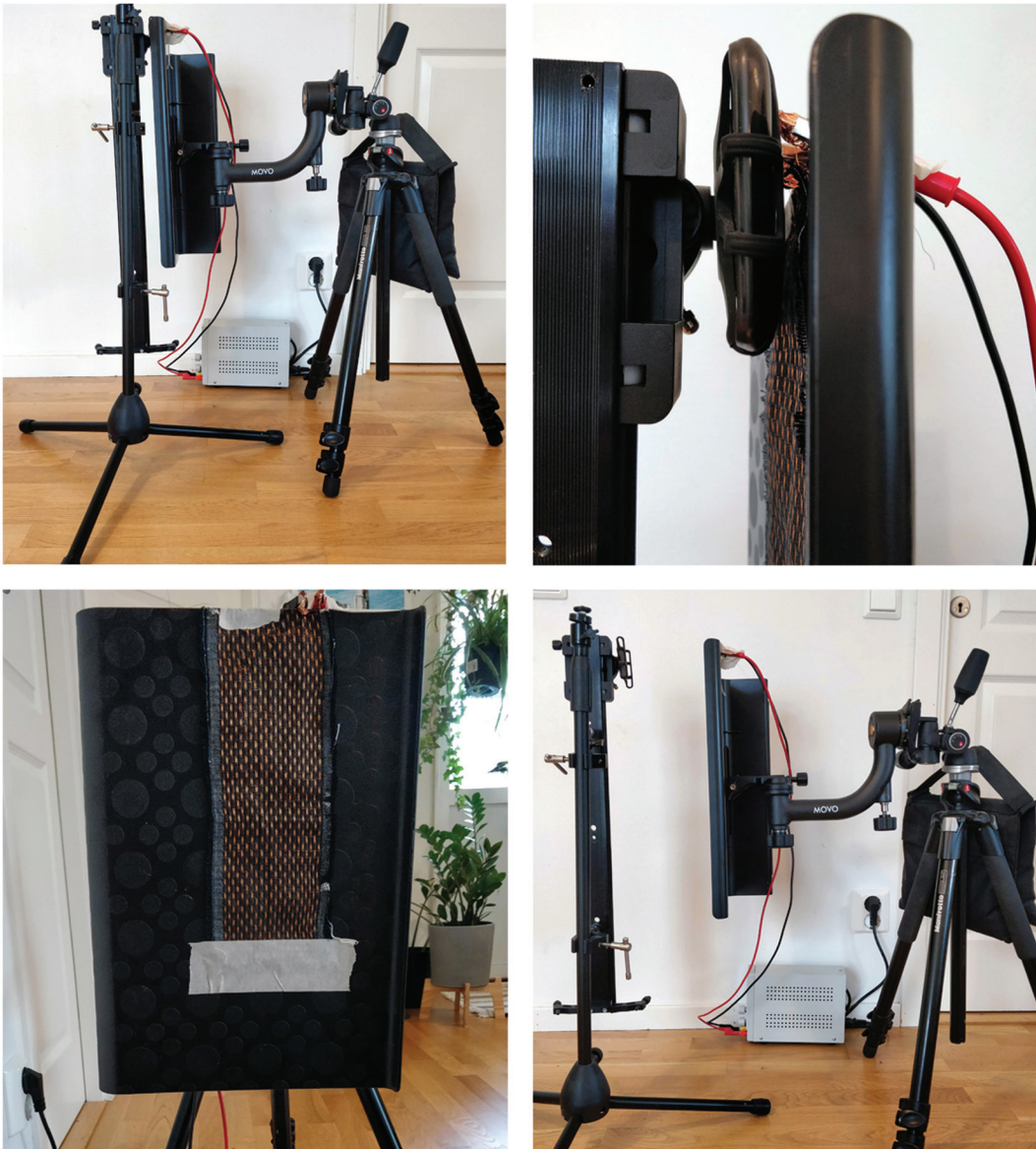
Figure 5: Full setup, sensing position (top left); detail sensing position (top right); textile suspension (bottom left); two tripods separated (bottom right). © Erin Lewis (2021).
