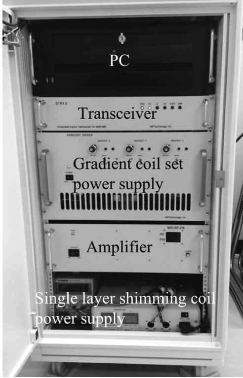
Fig. 6. Appearance of the MRI console The console consists of a PC, power supply for the G and SLS coils, amplifier, and transceiver for the NMR signal.
