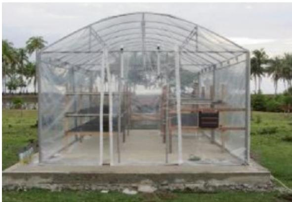
**Figure 7.** Force convection greenhouse solar dryer (Martunis, 2013).
