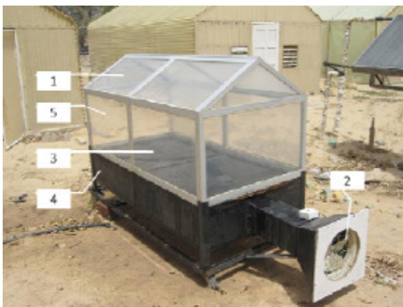
**Figure 3.** Indirect forced convection solar dryer; 1: Vent , 2: Exhaust fan , 3: Heating chamber, 4: Drying chamber and 5: Glass cover with fibre (Singh et al., 2017).
