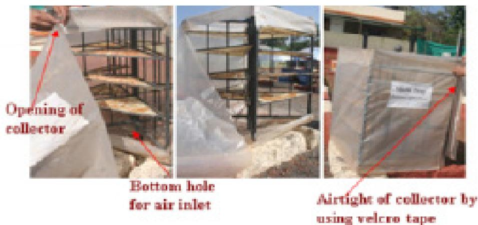
**Figure 5.** Low cost passive solar dryer (Sengar et al., 2009).
