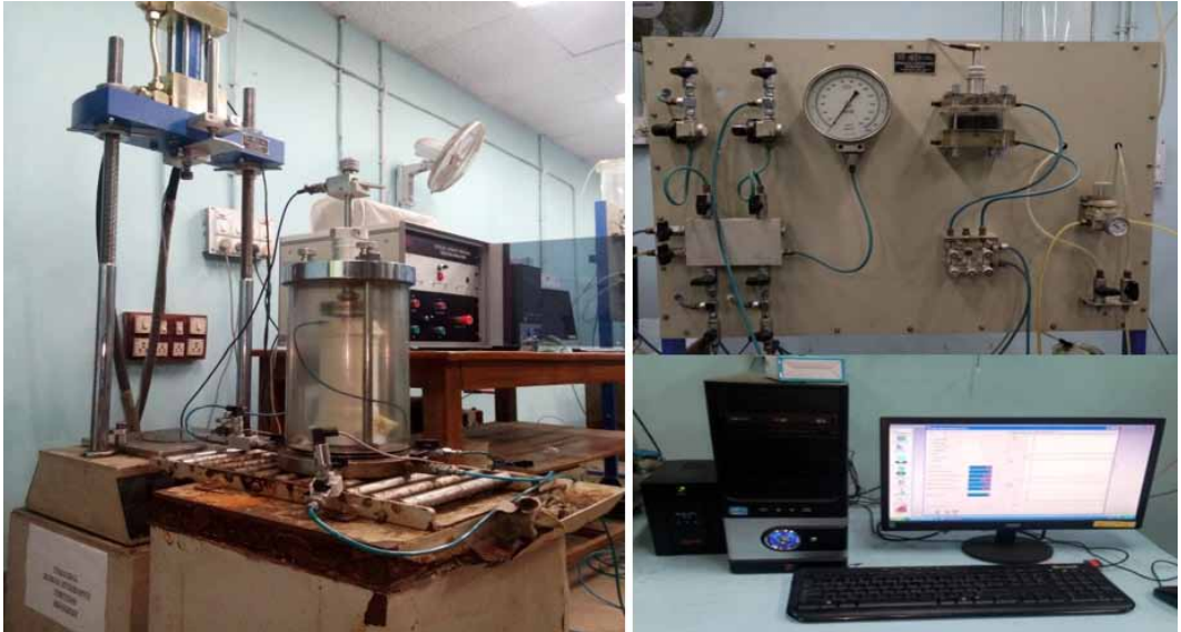
Figure 2. The laboratory cyclic triaxial test setup
