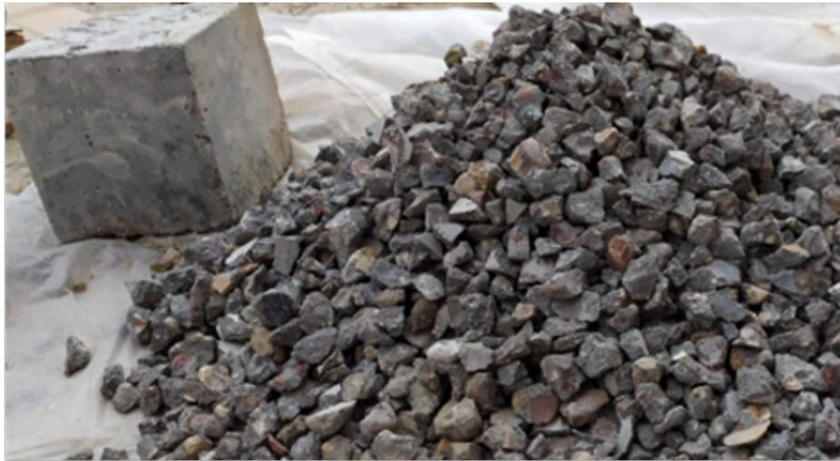
**Figure 2.** Recycled Concrete Aggregates (RCA)
