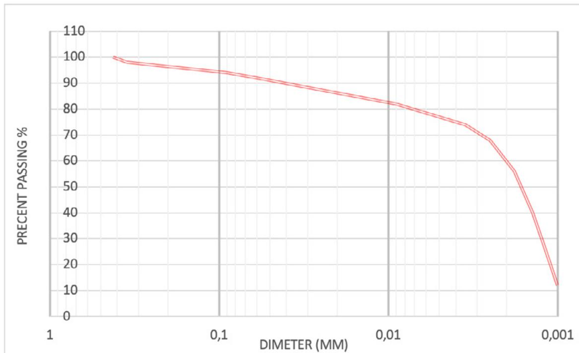
**Figure 1.** Grain size distribution of Soft clay
