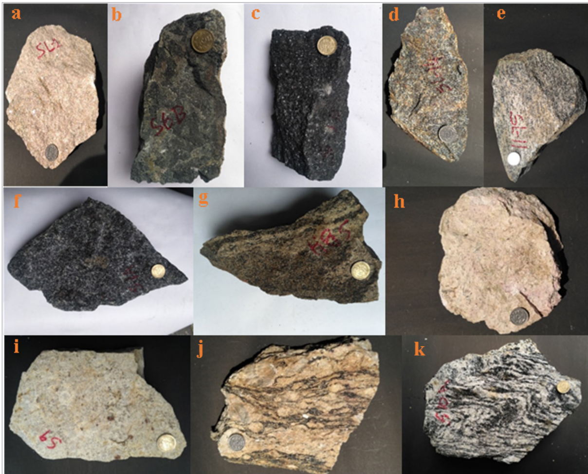
Figure 2. Rock samples collected from Sittampundi ultramafic terrain for mineralogical studies, chemical analysis and spectral measurements. (a) Pink granite, (b) pyroxenite, (c) gabbro, (d) meta-gabbro, (e) anorthosite, (f) pyroxenite, (g) meta-anorthosite, (h) pegmatite, (i) granite, (j) HBG and (k) migmatite.
