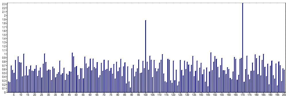
Fig. 3. MaxAE (9) for the best ARIMA models of 200 time series by (14), (15),  $T_0 = 84$  and  $T_{\text{forec}} = 168$  (fig. 1)
