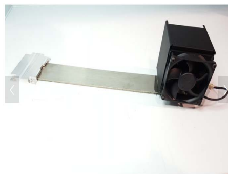
Fig. 14 FP OHP Air cooled microchip heat sink
