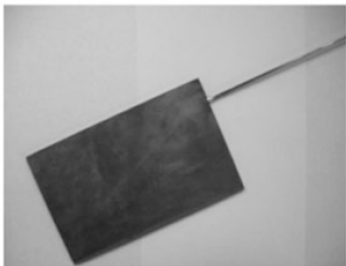
Fig. 11 FP OHP embeded with two layes of channel configuration
