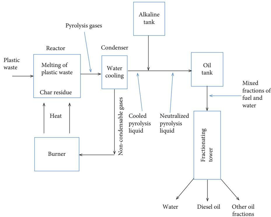
FIGURE 5: Plastic pyrolysis design flow diagram (authors' conceptualization).
