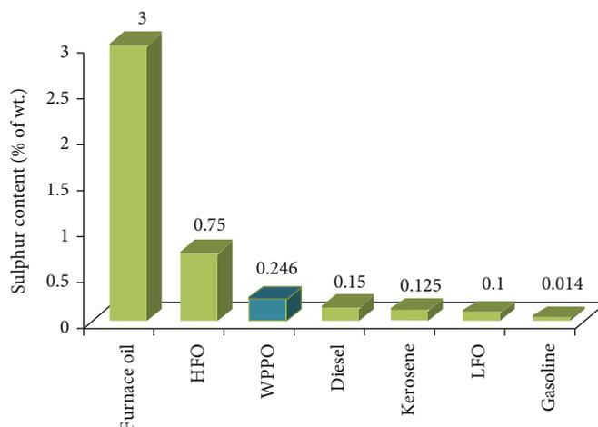
FIGURE 3: Sulphur content for various oils [6].
