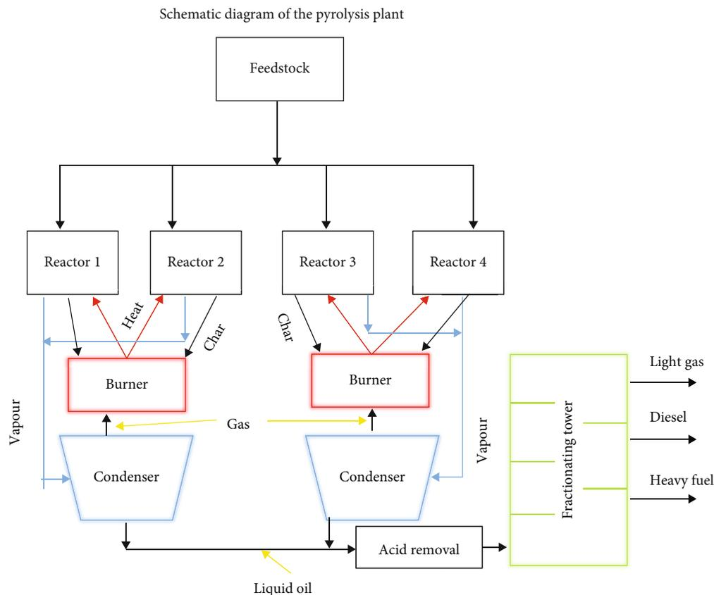
FIGURE 7: Four reactors arranged in parallel.
