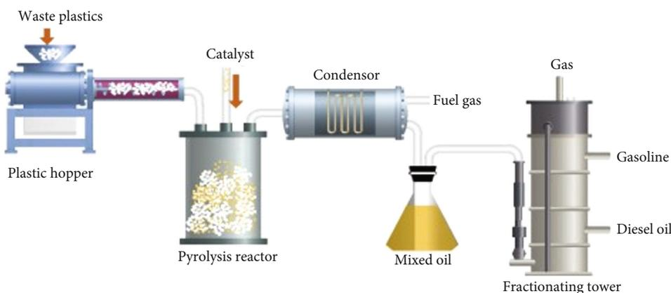
FIGURE 2: Plastic pyrolysis process description [5].
