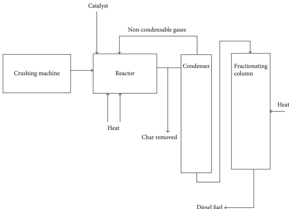
FIGURE 4: Overall process flow diagram.
