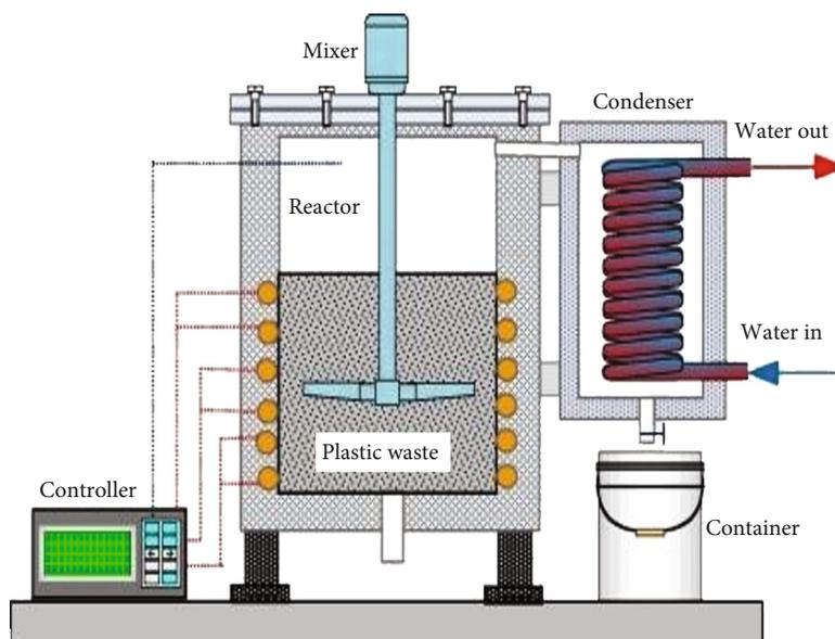
FIGURE 6: Internal view of pyrolysis reactor.
