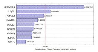
Figure 3. Pareto chart of standardized effects for SPF response. (2)OMC = Octyl methoxycinnamate , L= Linear, (1)GSO = Grape seed oil, (3)AVO = Avobenzone, Q = quadratic
