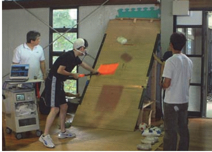
Fig. 2. Multistage shoveling test. The shoveling workload was expressed as the product of shoveling load (kg) by shoveling rate (times \text{min}^{-1} ).
