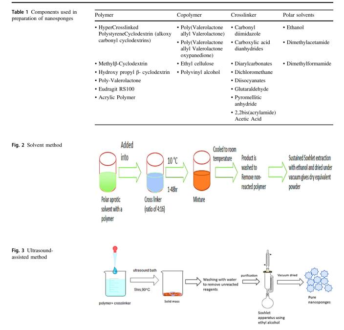
Excess amount of bi-distilled water was added to obtain the product from the above-cooled solution and the product was recovered under vacuum filtration (Fig. 2).
