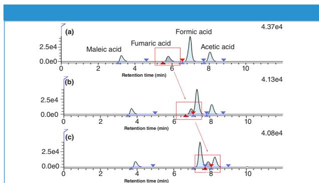
**Figure 1:** Chromatogram for each analytical condition. (a). Column temp.: 50 °C, B conc.: 10%. (b). Column temp.: 50 °C, B conc.: 30%. (c). Column temp.: 35 °C, B conc.: 40%.
