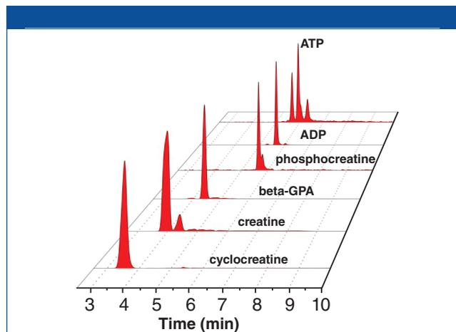
**Figure 3:** MRM chromatograms from a skeletal muscle extract (10× diluted with 50% methanol). Column: 50 × 2.1 mm iHILIC-(P) Classic. Elution: Gradient 3.
