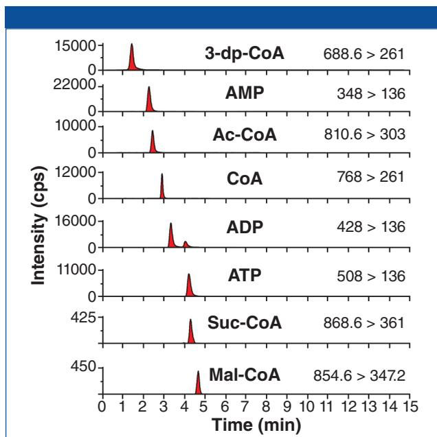
**Figure 1:** MRM chromatograms from 1 μM mixture of standards in 50% methanol. Column: 50 × 2.1 mm iHILIC-(P) Classic. Elution: Gradient 2.
