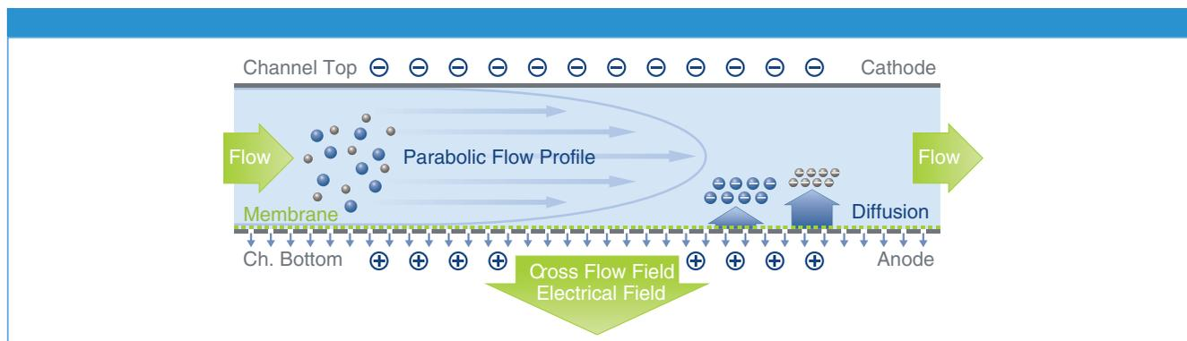
**Figure 2:** Schematic of the fractionation in an EAF4 channel both by size and surface charge.
