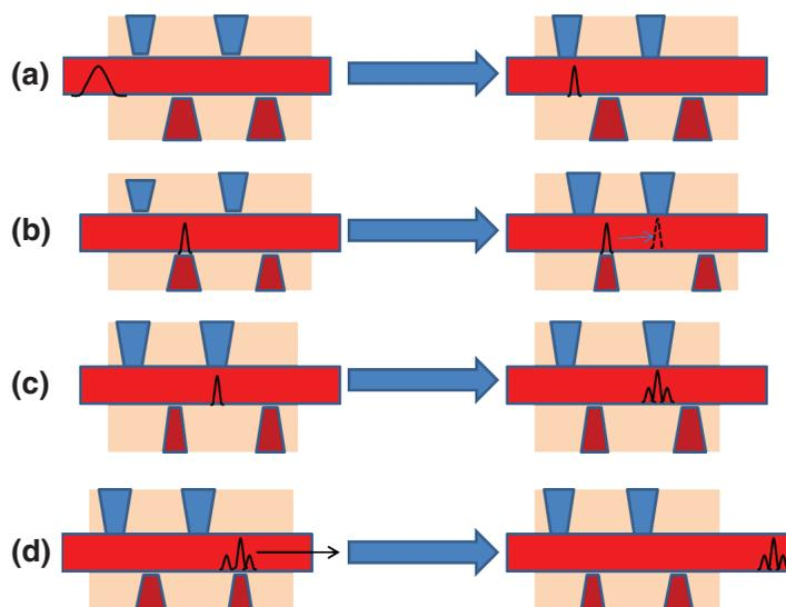
that both connects the columns and transfers the first-dimension column effluent into the second-dimension column effluent will act as the heart of multidimensional chromatography. Like the inlet on a traditional gas chromatograph, the modulator must collect a chosen aliquot of the first-dimension effluent, focus it into
