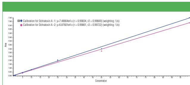
**Figure 2:** Calibration curve example: Ochratoxin A. A 7-point calibration curve prepared at 0.5, 1, 5, 10, 25, 50, and 100 ng/mL.
