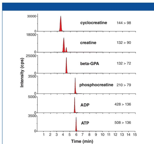
**Figure 2:** MRM chromatograms from 1 μM mixture of standards dissolved in 50% methanol. Column: 50 × 2.1 mm iHILIC-(P) Classic. Gradient program 3. Phosphocreatine detected in negative ESI.
