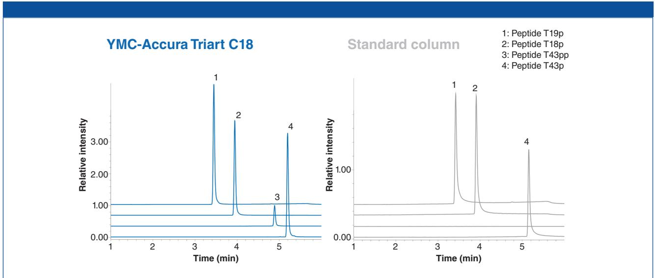
**Figure 2:** Extracted ion chromatograms (EICs) of phosphopeptide mixture separated with the bioinert YMC-Accura Triart C18 column and the stainless-steel column hardware equilibrated with 10 injections.
