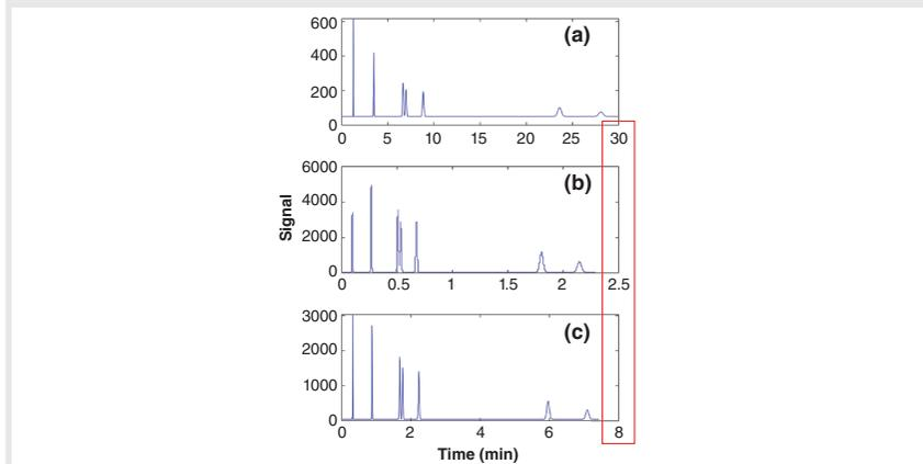
**FIGURE 2:** (a–d) Effect of mobile phase concentration of organic solvent on elution pattern for a simple mixture. The mixture is full resolved (five peaks) when mobile phases with either 40 or 60% acetonitrile (ACN) are used; however, the separation with 60% acetonitrile is clearly more desirable because the analysis is complete in a much shorter time. The red star in (b) indicates two compounds are coeluted.
