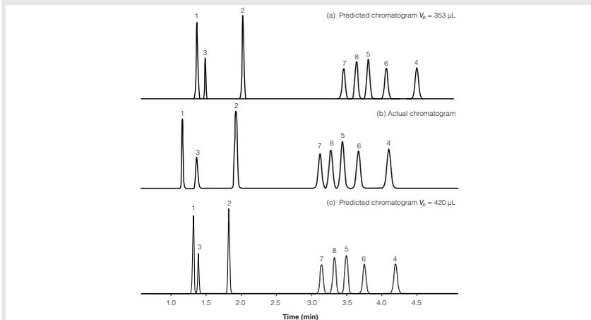
**FIGURE 6:** Effect of the difference in the initial %B to that used to construct the model on the retention time accuracy of the final optimized condition.
