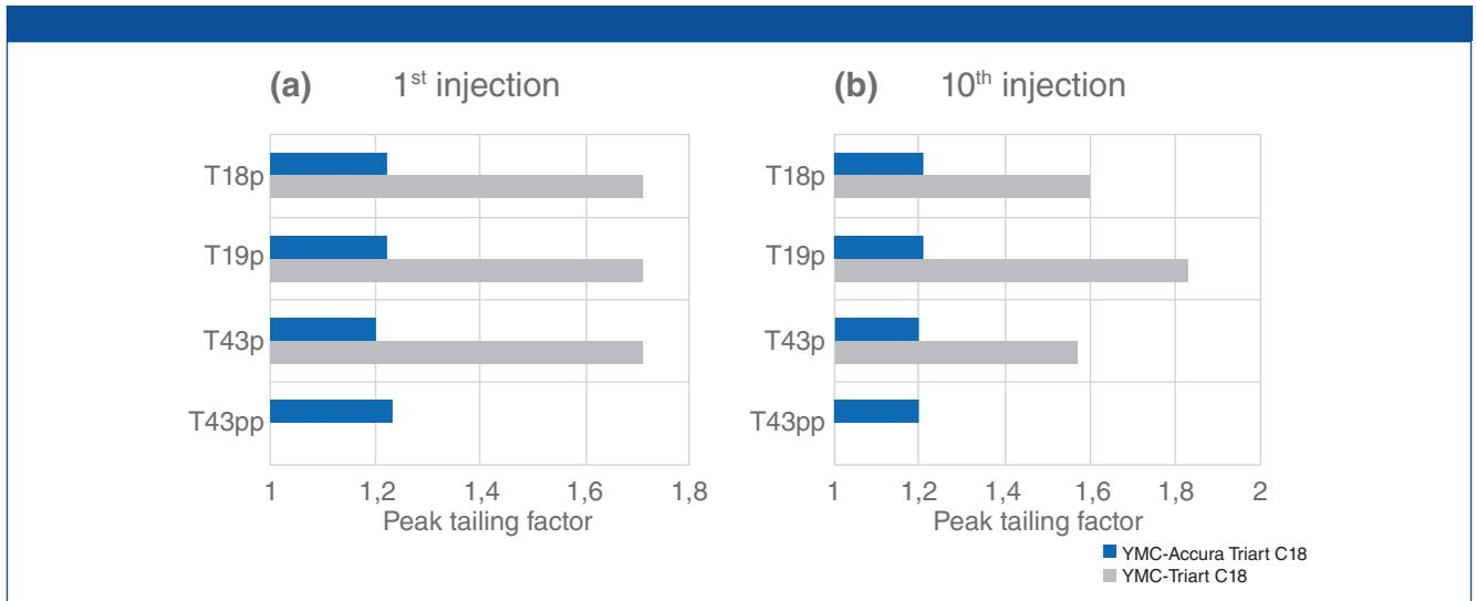
**Figure 3:** Peak tailing factor of the four phosphopeptides analyzed by the bioinert YMC-Accura Triart C18 column (blue) and the stainless-steel standard column (grey) after (a) the first injection and (b) the tenth injection.
