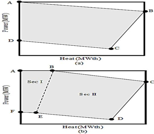
Fig. 3. Heat-power feasible operation region of a CHP unit
