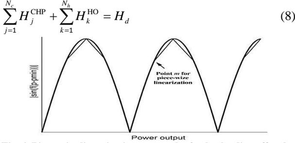
Fig. 4. Piece-wise linearization approach of valve loading effect by four linear segments for a sample unit
