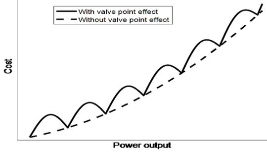
Fig. 2. Comparison of cost function with valve effect and that without valve effect
