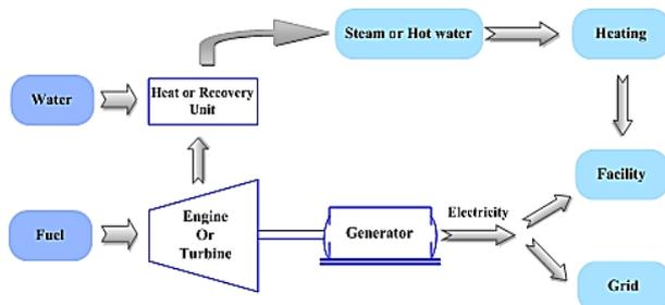
Fig. 1. Common configuration of a CHP
