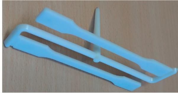
FIGURE 1: Injection molded part from the two-cavity mold including the runner system and the two tensile specimens.
