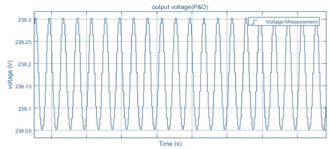
Figure 12: O/P voltage ripple of KY converter with P&O algorithm
