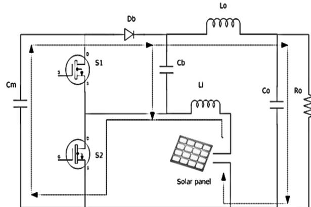
Figure 3: Circuit diagram represents the power flow via KY converter in mode 1
