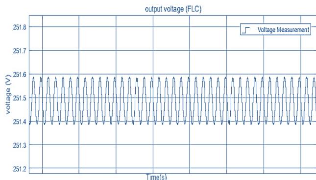
Fig.11: O/P voltage ripple of KY converter with a fuzzy logic controller
