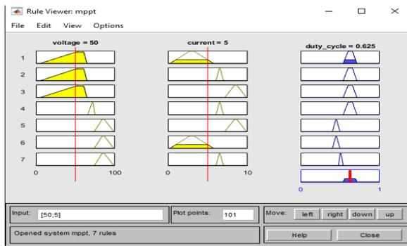
Figure 5(b). Rule viewer of the fuzzy logic controller for KY converter
