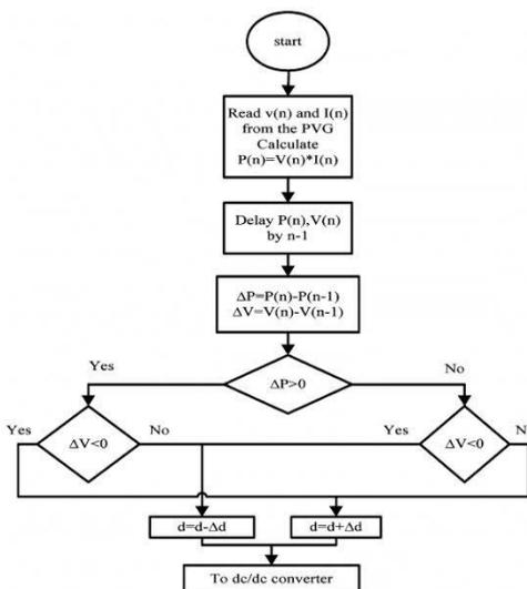
Figure 6: P&O algorithm used for KY converter
