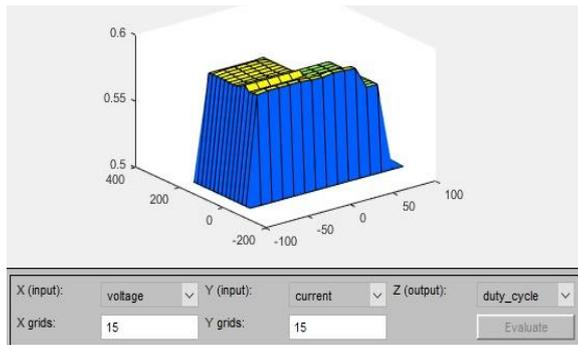
Figure 5(c): Surface view of the fuzzy logic controller for KY converter
