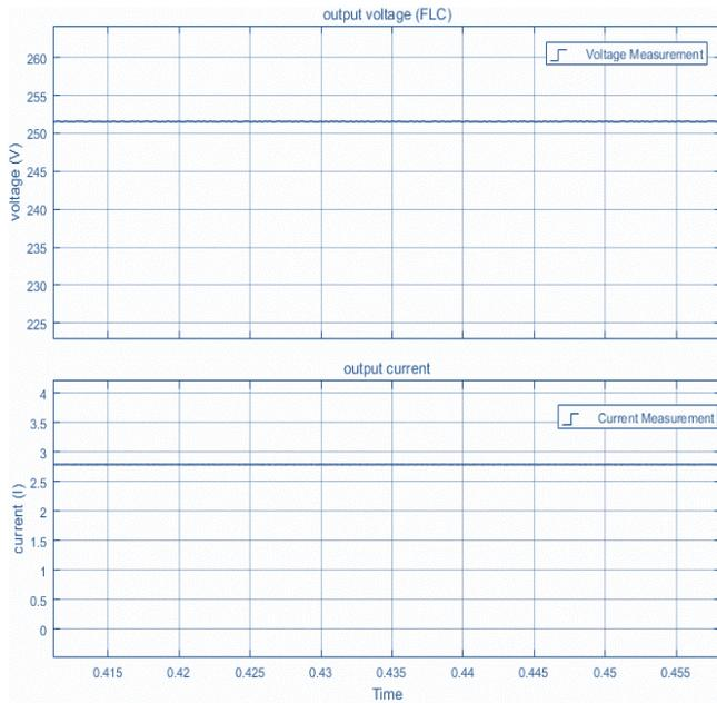
Figure 9: O/P of KY converter with fuzzy logic controller
