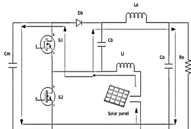
Figure 4: Circuit diagram represents the power flow via KY converter in mode 2
