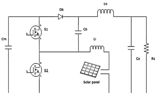
Figure 2: Circuit illustration of KY converter
