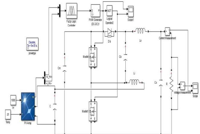
Figure 7: KY converter simulation with fuzzy logic controller
