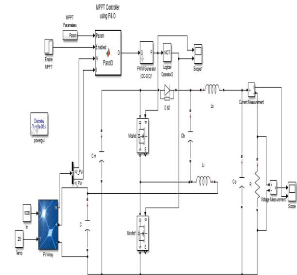
Figure 8. Simulation of KY converter with P&O algorithm
