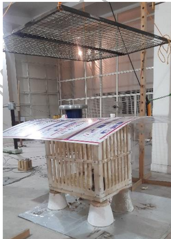
Figure 1. The presence of monkey's cage under a uniform electrical field of 3 kV/m.
