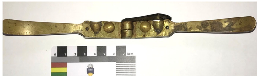
Figure 8. A of .36 bullet mould for the Colt revolver from the Glenroy NMP camp (Photograph: Tony Pagels).
