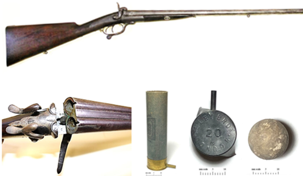
Figure 9. (top) Westley Richards & Co. breech loading double-barrel carbine, 20g with Lefauchaux-action and ammunition; and (bottom L–R) the action opened to illustrate the design of the drop breech and slot in the top of the barrel to accommodate the pin of the cartridge; a 20-gauge pinfire cartridge with brass head and cardboard body; used brass pinfire cartridge head; unused 20-gauge lead ball. Scale in mm (Photographs: Tony Pagels).
