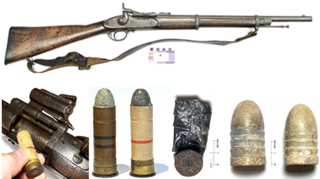
Figure 10. (top) Snider-Enfield artillery carbine MkIII, manufactured by P. Webley & Son and marked Q↑G on the lockplate. (Queensland Museum uncatalogued); and (bottom L-R) loading a Boxer cartridge into the carbine; unused MkVIII and MkIX Boxer cartridges; used Boxer cartridge recovered from Eyre's Creek NMP camp; Type 6 bullet with four cannelures as used in the MkVIII cartridge; Type 7 bullet with three cannelures as used in the MkIX cartridge. Scale in mm (Photographs: Tony Pagels).
