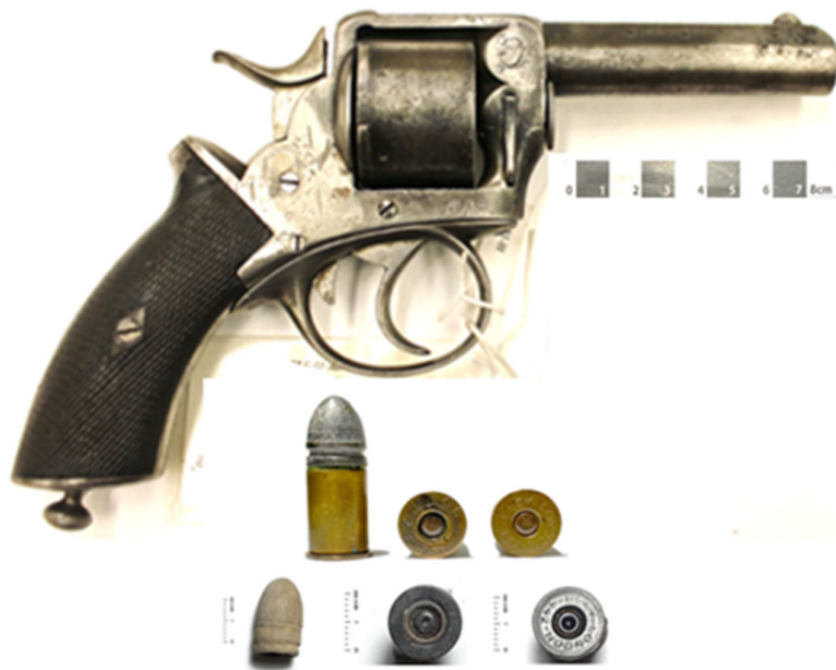
Figure 15. (top) P. Webley & Son R.I.C No. 3 Second Pattern revolver, with frame marked ‘C.I.B. 1005’, and ↑over Q.G. (Queensland Museum H1909); (centre, L–R) .442-inch cartridges for the P. Webley & Son RIC revolver, a pre-1874 Boxer constructed, battery primed cartridge with headstamp ‘ELEY BROS’ and a post-1874 cartridge with the headstamp ‘ELEY .442 LONDON’; and (bottom L–R) .442 bullet, base of a pre-1874 .442 cartridge, and base of a post-1874 .442 cartridge. Scale in mm (Photographs: Tony Pagels).
