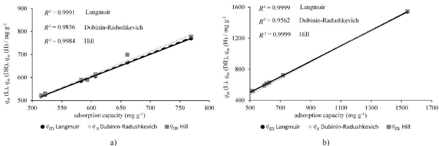
Fig. 5 – Correlation between adsorption parameters ( $q_m$  from Langmuir,  $q_s$  from Dubinin-Radushkevich,  $q_m$  from Hill) and adsorption capacities ( $q_e$ ) obtained experimentally a) at different temperatures; b) at different pH values (adsorption capacities obtained in the experiment with the initial concentration of 150 mg L<sup>-1</sup> in the reaction solution)
