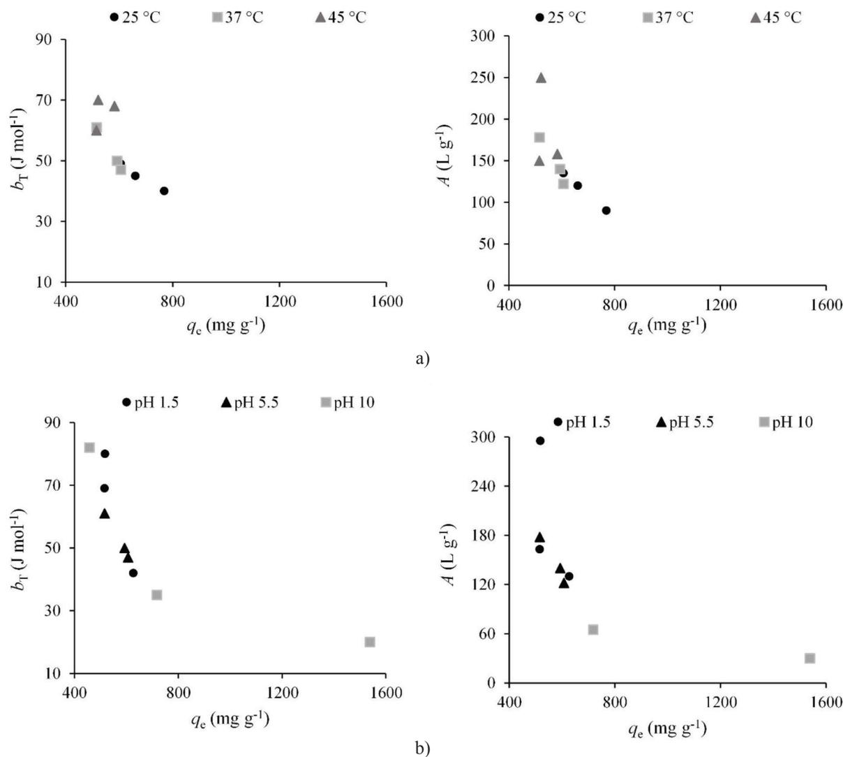
Fig. 4 – Relationship between Temkin adsorption parameters ( $b_T$  and  $A$ ) and the adsorption capacity  $q_e$  a) at different temperatures; b) at different pH values (adsorption capacities obtained in the experiment with the initial concentration of 150 mg L<sup>-1</sup> in the reaction solution)
