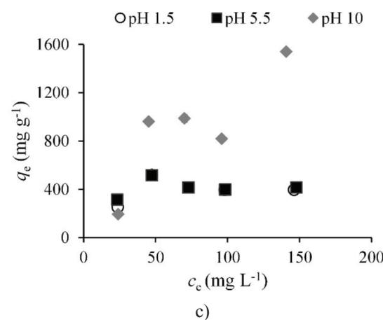
Fig. 2 – Data for adsorption isotherms ( $q_e$  vs  $c_e$  diagrams) at 25, 37, and 45 °C (pH 5.5). Data shown are means  $\pm$  standard deviation of means. a) *p*-coumaric acid; b) caffeic acid; c) chlorogenic acid.
