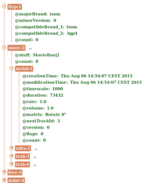
Fig. 14.1 Representation of a fragment of an MP4-like video container, of an original video acquired by a Samsung Galaxy S3
