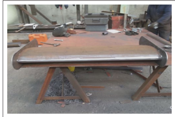
Figure 6. Hydrofoil during fabrication in Arklow Marine Services (see Note 2).
