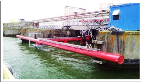
Figure 9. Test apparatus (grey, shown on left) fitted to Tocardo (See Note 3) beam (red) at TTC (See Note 1).
