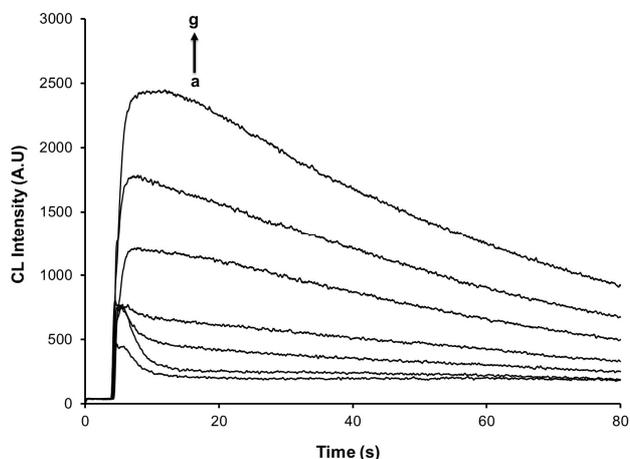
**Fig. 5.** Typical CL time profiles of remifentanyl. a) blank, b) 1.75, c) 18.23, d) 36.46, e) 72.92, f) 109.39 and g)  $182.32 \mu\text{g ml}^{-1}$ .
