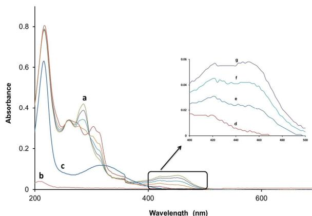
**Fig. 6.** UV-Vis absorption spectrum a) Ru(phen)<sub>3</sub><sup>2+</sup> 1.0 × 10<sup>-5</sup> M, b) Remifentanyl 0.72, c) Cerium(IV) 3.3 × 10<sup>-5</sup> M in 3.3 × 10<sup>-3</sup> M sulfuric acid and d-g) spectra of mixture of Ce(IV)-Ru(phen)<sub>3</sub><sup>2+</sup>-remifentanyl, 3 to 12 min after mixing and time intervals of 3 min.
