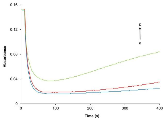
**Fig. 7.** Changes in concentration and absorption of  $\text{Ru}(\text{phen})_3^{2+}$  complex over time a) in the mixture of  $\text{Ru}(\text{phen})_3^{2+}$ -Cerium(IV) b and c) in the mixture of  $\text{Ru}(\text{phen})_3^{2+}$ -Cerium(IV)-remifentanyl,  $\text{Ru}(\text{phen})_3^{2+}$ :  $6.6 \times 10^{-6}$  M,  $\text{H}_2\text{SO}_4$ :  $3.3 \times 10^{-3}$  M, Cerium(IV):  $3.3 \times 10^{-5}$  M, remifentanyl: b)  $72.92 \mu\text{g ml}^{-1}$ , c)  $187.32 \mu\text{g ml}^{-1}$ .
