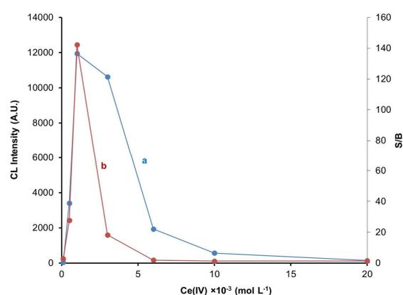
**Fig. 3.** Optimization of cerium(IV) concentration. a) CL of remifentanyl (S) at different concentrations of cerium(IV) b) S/B ratio. Remifentanyl  $145.85 \mu\text{g ml}^{-1}$ ,  $\text{Ru}(\text{phen})_3^{2+}$ :  $1.0 \times 10^{-3}$  M,  $\text{H}_2\text{SO}_4$ : 0.1 M.
