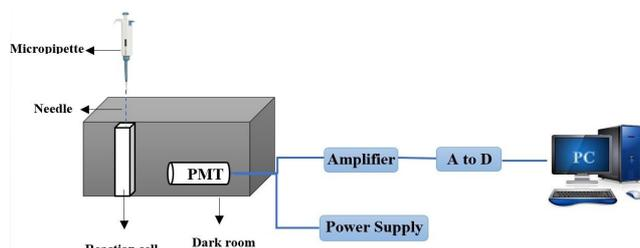
**Fig. 2.** The schematic view of the CL instrument.
