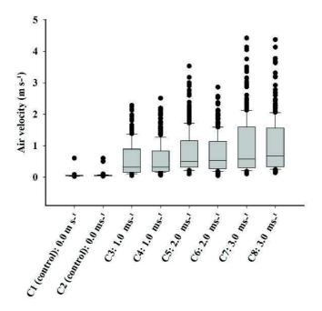
**Figure 4.** Boxplot of air velocity measurements at 275 locations in two replicate cages in still air and 3 controlled velocities. C1 and C2) Control (cages 1 and 2, still air), 0 m s<sup>-1</sup>; C3 and C4) Cages 3 and 4, set point 1 m s<sup>-1</sup>; C5 and C6) Cages 5 and 6, set point 2 m s<sup>-1</sup>; C7 and C8) Cages 7 and 8, set point 3 m s<sup>-1</sup>.
