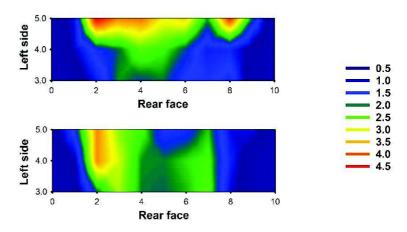
**Figure 6.** Velocity distribution map for the front feeding zone at the two bottom levels in Cage 8 with velocity set point 3 m s<sup>-1</sup>; A) lowest level, Z0; B) bird head level, Z1.
