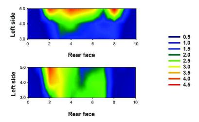
**Figure 5.** Velocity distribution map for the front feeding zone at the two bottom levels in Cage 7 with velocity set point 3 m s<sup>-1</sup>; A) lowest level, Z0; B) bird head level, Z1.
