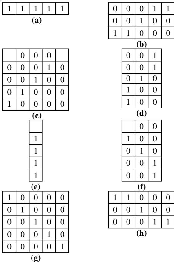
Fig. 3 Structure Elements Eight Direction (a) Strell line  $0^{\circ}$  (b) Strell line  $22.5^{\circ}$  (c) Strell line  $45^{\circ}$  (d) Strell line  $67.5^{\circ}$  (e) Strell line  $90^{\circ}$  (f) Strell line  $112.5^{\circ}$  (g) Strell line  $135^{\circ}$  (h) Strell line  $157.5^{\circ}$
