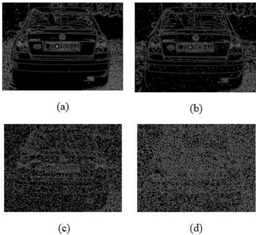
Fig. 11 First group of images resulted from Canny edge detection using Greek car images with different levels (a) Without Salt and pepper noise (b) Salt and pepper noise level 0.2 (c) Salt and pepper noise level 0.4 (d) Salt and pepper noise level 0.6.
