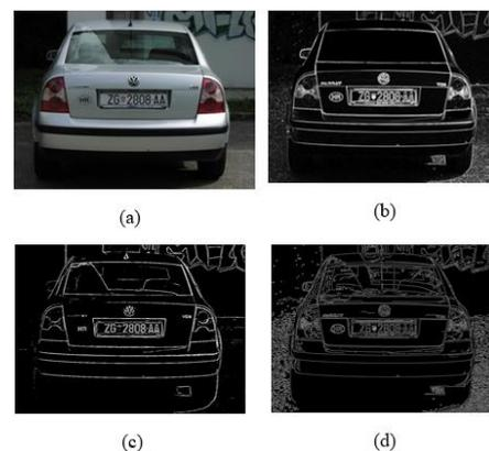
Fig. 6 First group from Greek car images of edge detection experiments with different algorithms (a) Color image (b) Ground truth image (c) Result by using Mathematical Morphology (d) Results by using Canny operator
