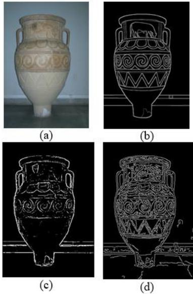
Fig. 7 Second group from Berkeley images of edge detection experiments with different algorithms (a) Color image (b) Ground truth image (c) Result by using Mathematical Morphology (d) Results by using Canny operator
