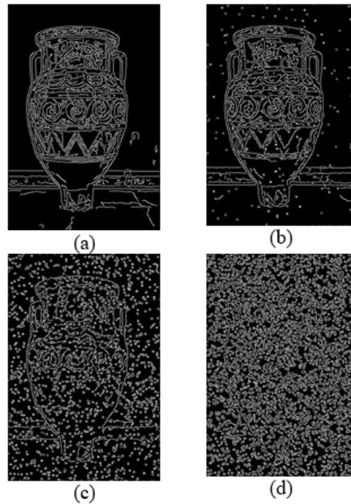
Fig. 13 A second group of images resulted from Canny edge detection using Berkeley images with different levels (a) Without Salt and pepper noise (b) Salt and pepper noise level 0.2 (c) Salt and pepper noise level 0.4 (d) Salt and pepper noise level 0.6
