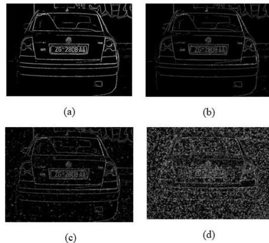
Fig. 10 First group of images resulted Mathematical Morphology edge detection from Greek car images with different levels (a) Without Salt and pepper noise (b) Salt and pepper noise level 0.2 (c) Salt and pepper noise level 0.4 (d) Salt and pepper noise level 0.6
