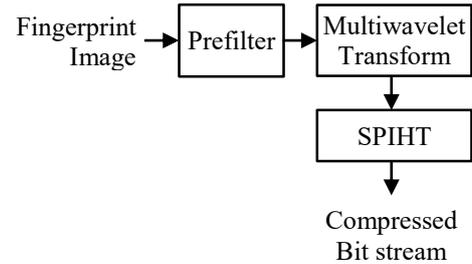
Fig.1(a). Block diagram for general fingerprint image compression
