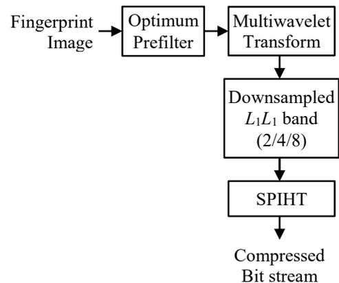
Fig.1(b). Block diagram for the proposed fingerprint image compression
