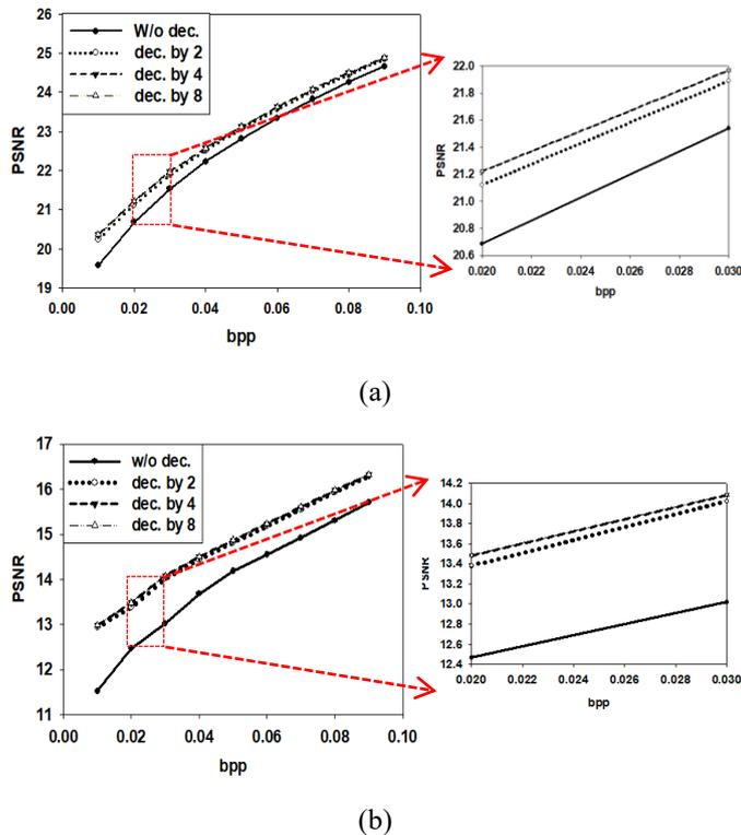
Fig.3. Average PSNR at lower bit rates with an inset showing the PSNR in between bit rates 0.02 and 0.03 for the images in (a) NIST database (b) NITGEN database
