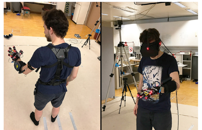
Fig. 10. Left: a person wearing the recording equipment (Phase-Space glove and Perception Neuron). Right: a person testing the application in a VR environment with an Oculus HMD.
