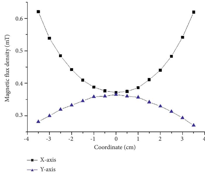
FIGURE 5: Measured line profile of modulation magnetic field peak-to-peak amplitude along the X- and Y-axis. The X-axis is in the direction of the main magnetic field, and the Y-axis is in the horizontal plane between poles.
