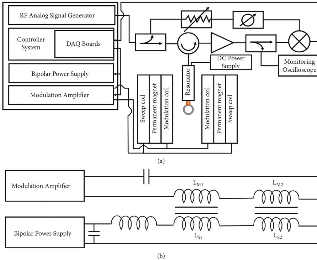
FIGURE 2: EPR spectrometer connection. (a) A schematic of EPR spectrometer for *in vivo* tooth dosimetry. (b) Circuit connection of modulation coils ( $L_{M1}$  and  $L_{M2}$ ) and sweep coils ( $L_{S1}$  and  $L_{S2}$ ). LC series resonant is used to operate the modulation coils with 21.2 kHz. In sweep coil circuitry, LC low-pass filter is connected to block the AC induced by the AC magnetic field from the modulation coil.
