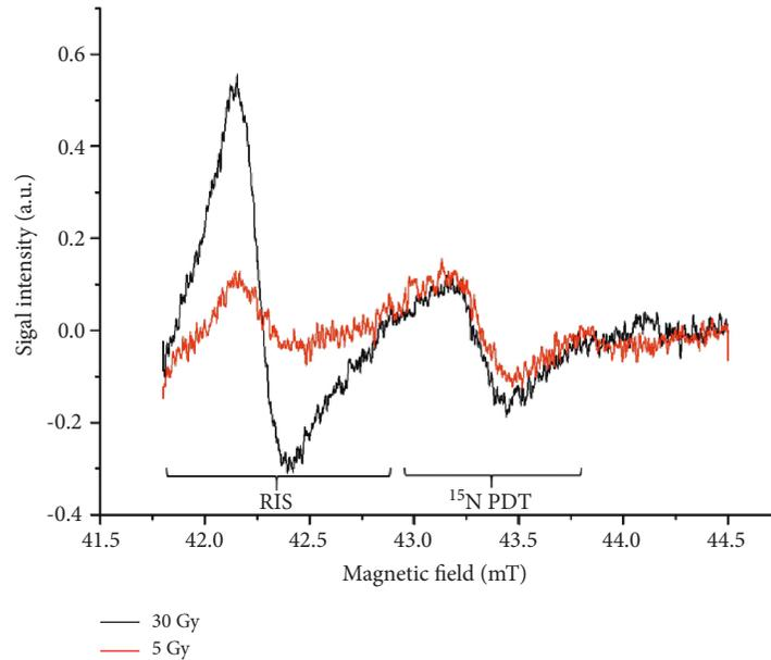
FIGURE 7: Measured EPR spectrum. Spectrum acquired from 5 (red) and 30 Gy irradiated incisors. Two peaks are shown in each spectrum. RIS of the tooth (left peak) is distinguishable in amplitude. The reference material,  $^{15}\text{N}$  PDT (right peak), has the same height in both spectra.
