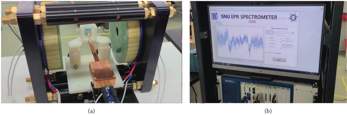
FIGURE 6: Spectrum acquisition with the developed magnet system: (a) EPR spectra are acquired with a surface coil resonator at the center of the magnet system and (b) the measured signals are collected with the controller system, and the EPR spectrum is acquired.
