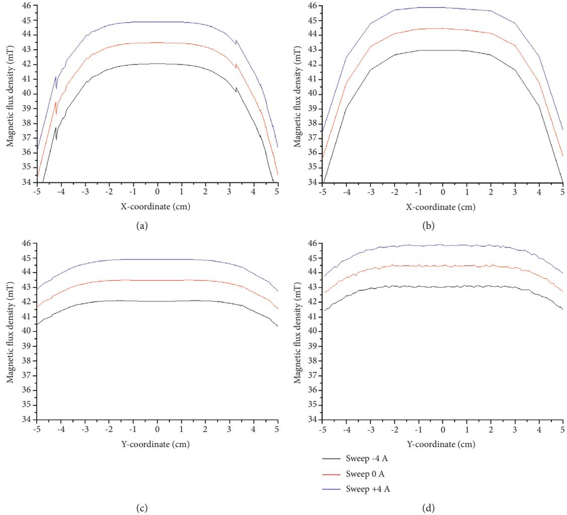
FIGURE 4: Measured profiles of magnetic flux density along the X- and Y-axis. (a) X-axis profile of FEM results with and without current in sweep coils; (b) X-axis profile of measurement; (c) Y-axis profile of FEM result; (d) Y-axis profile of measurement result. It should be noted that the direction is on the X-axis, and the XY plane is a horizontal midplane between the pole faces.
