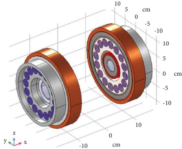
FIGURE 1: A schematic design of EPR magnet system for *in vivo* tooth dosimetry: the magnet system typically comprises PMs (blue), sweep (brown), and modulation coils (red). It should be noted that the direction of the main magnetic field is on the X-axis.
