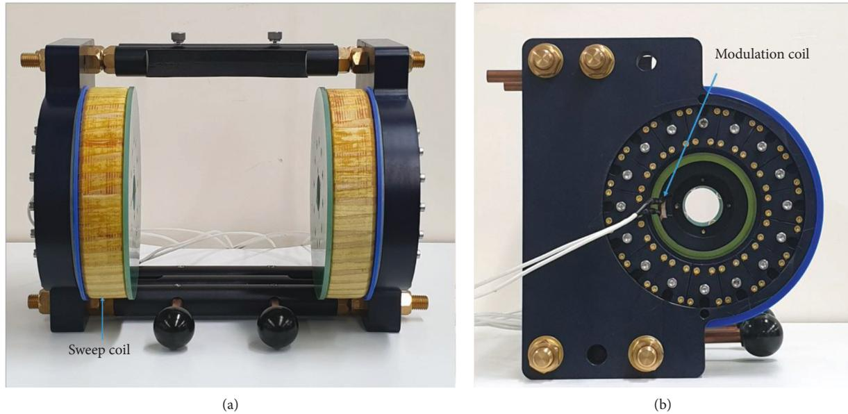
FIGURE 3: Manufactured magnet system for *in vivo* EPR tooth dosimetry. PMs are invisible from the outside. (a) Sweep coils are exposed from the front view. (b) Parts of the modulation coils and their wiring are shown from the side view.
