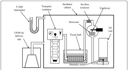
**Figure 1 Schematic representation of the apparatus set up within the incubator.** Bellows of transport ventilator shown in extended position and slave bellows in compressed state. Exhalation phase occurs when transport ventilator bellows compress. Bovine trachea immersed in physiological salt solution within tissue bath. Pressure augmentation supplied by CPAP air delivery unit is connected to sealed incubator cabinet.
