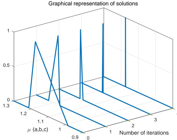
Figure 2. Graphical representation of accelerated solutions  $\hat{\mu}_n$  by LFR Aitken's method
