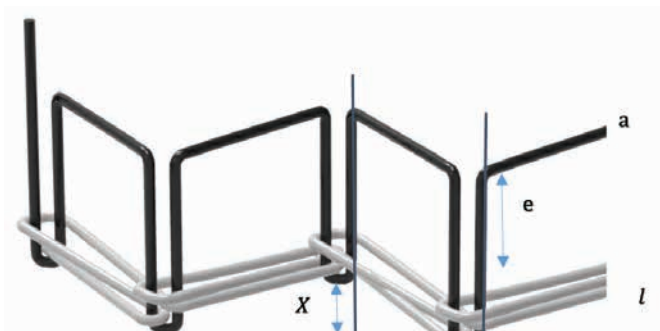
Figure 4. Geometrical model of chain stitch type 404.
