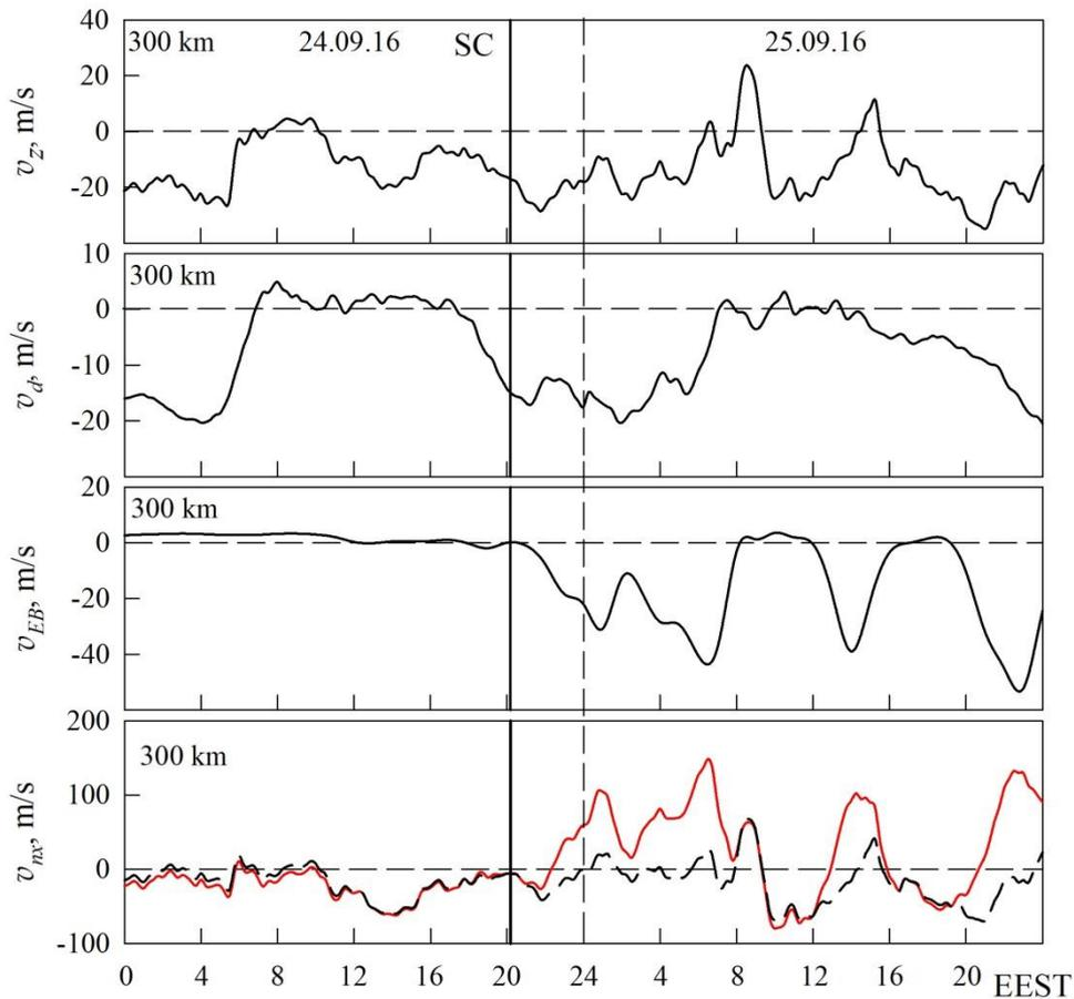
**Fig. 3.** Temporal variations in the vertical component of the plasma transport velocity  $v_z$  (Kharkiv ISR experimental data), the plasma transport velocity due to ambipolar diffusion  $v_d$  (calculation), the plasma transport velocity due to electromagnetic drift  $v_{EB}$  (calculation) and meridional neutral wind velocity  $v_{nx}$  (calculation) during the magnetic storm on September 25, 2016 and reference day on September 26, 2016 at the altitude of 300 km
