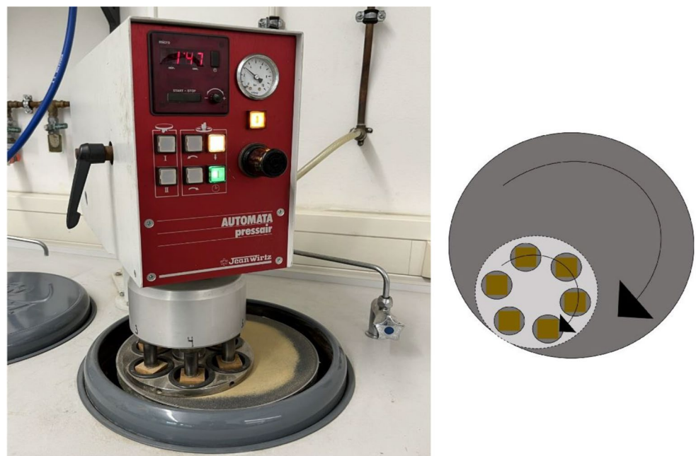
Fig. 3 Left: Disc grinding machine (Jean Wirtz -type: Polo 250/2) with wood samples. Right: Schematic diagram showing the direction of rotation of the grinding disc (dark grey), sample holder (light grey) and samples (brown) in synchronous mode
