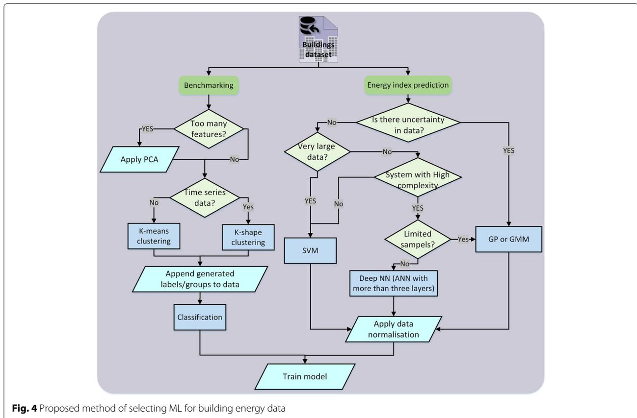
**Fig. 4** Proposed method of selecting ML for building energy data
