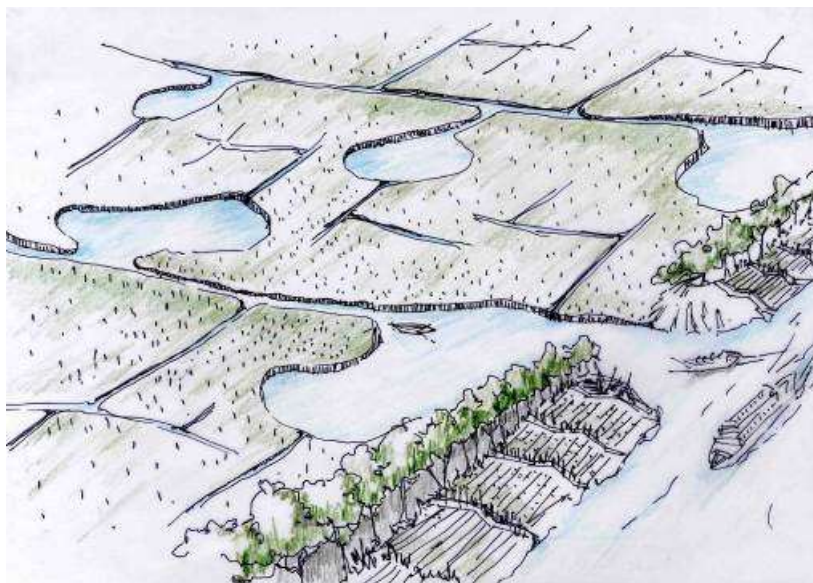
Figure 18: System of flood pockets, irrigation canals, lowlands, earthen dike as flood protection
