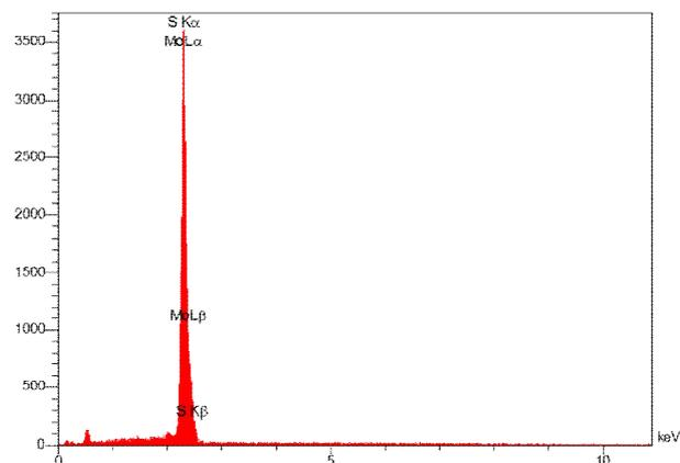
**Fig. 2.** The EDX spectrum of the MoS<sub>2</sub> nano-sheets.
