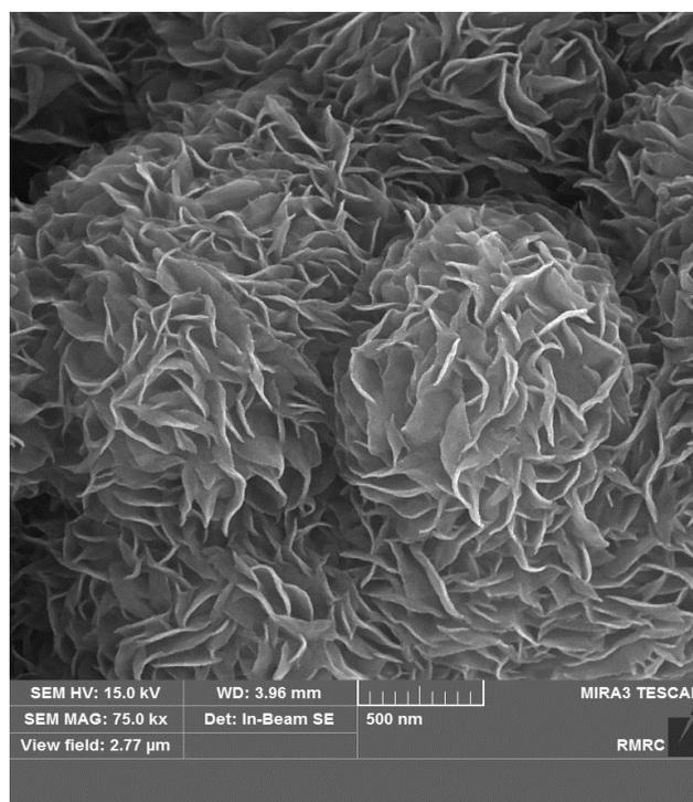
**Fig. 1.** The SEM image of the MoS<sub>2</sub> nano-sheets.
