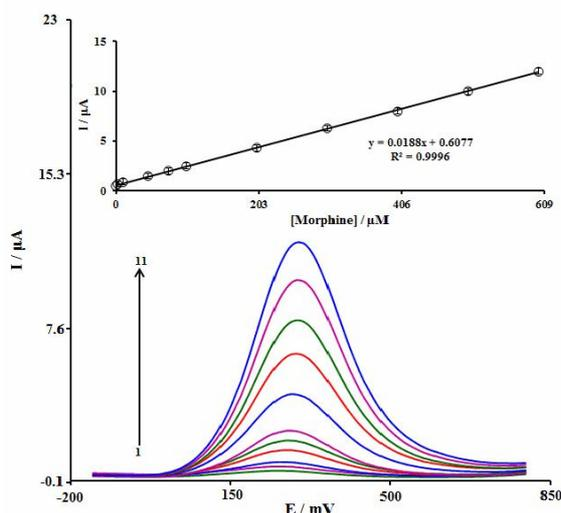
**Fig. 8.** DPVs obtained for MoS<sub>2</sub>NS<sub>S</sub>/SPE in 0.1 M PBS (pH 7.0) consisting of distinct concentrations of morphine. 1 to 11 corresponded to 0.05, 2.5, 10.0, 45.0, 75.0, 100.0, 200.0, 300.0, 400.0, 500.0, and 600.0 μM of morphine. Inset: The peak current plot as a function of concentration of morphine in a range between 0.05 and 600.0 μM.
