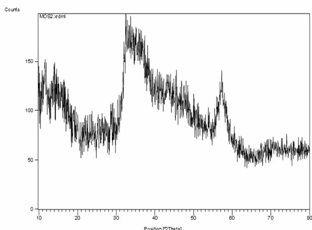
**Fig. 3.** The XRD pattern for the MoS<sub>2</sub> nano-sheets.
