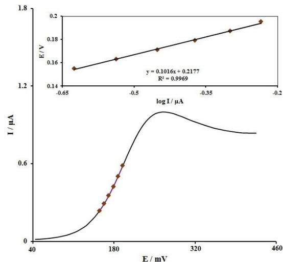
**Fig. 6.** LSV (at 10 mV s<sup>-1</sup>) of the electrode in 0.1 M PBS (pH of 7.0) consisting of 70.0 μM morphine. As seen, the points represent data utilized in the Tafel plot and inset represents Tafel plot derived from LSV.
