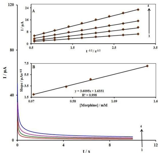
**Fig. 7.** Chrono-amperograms observed at MoS<sub>2</sub>NS<sub>S</sub>/SPE in 0.1 M PBS (pH = 7.0) for distinct concentrations of morphine. 1 to 4 corresponded to 0.1, 0.5, 0.8, and 1.5 mM of morphine. Inset a):  $I$  vs.  $t^{-1/2}$  plots achieved from chrono-amperograms 1-4. Inset b) The slope plot of the straight lines *versus* the concentration of morphine.
