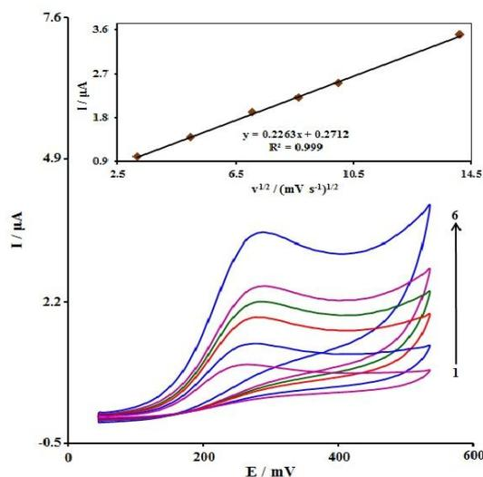
**Fig. 5.** CVs of MoS<sub>2</sub> NS<sub>s</sub>/SPE in 0.1 M PBS (pH of 7.0) containing 70.0 μM of morphine at diverse scan rates. 1 to 6 corresponded to 10, 25, 50, 75, 100, and 200 mV s<sup>-1</sup>. Inset shows changes in the anodic peak current *versus* the square root of the scan rate.
