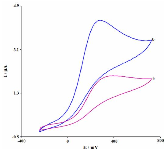
**Fig. 4.** The CVs of a. the bare SPE and b. the MoS<sub>2</sub> NS<sub>s</sub>/SPE in the presence of 200.0 μM of morphine at pH equal to 7.0. The scan rate has been 50 mV s<sup>-1</sup>.
