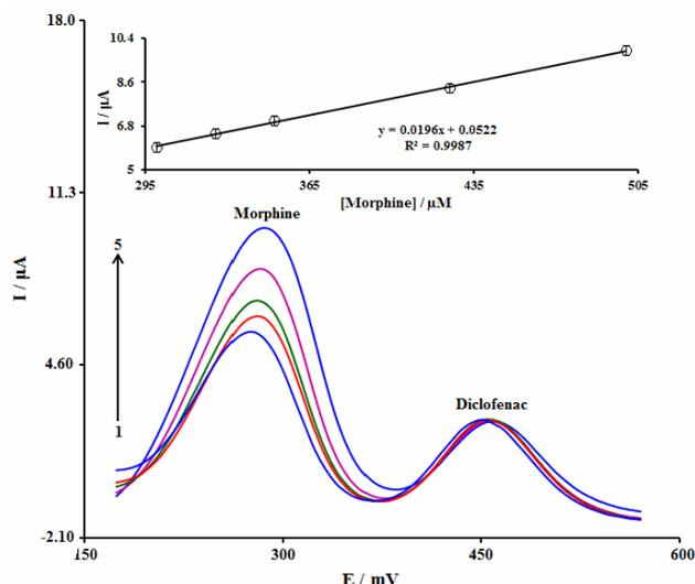
**Fig. 9.** DPVs observed for morphine at MoS<sub>2</sub> NS<sub>s</sub>/SPE in the presence of 150.0 μM diclofenac in 0.1 M PBS (pH = 7.0). Concentration of morphine (in a range between 1 and 5): 300.0, 325.0, 350.0, 425.0, and 500.0 μM.
