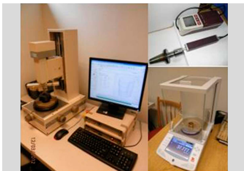
Figure 3 Devices used: MUK – F 300 PC, Mitutoyo SJ-201 and Voyager Pro VP 613 CN
