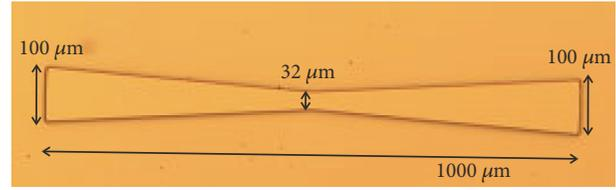
FIGURE 1: Light microscope image (top-view) of a confocal BAL resonator with a bow-tie-shaped laser ridge and, in this example, a  $32 \mu\text{m}$  wide constriction in the middle plane. The resonator length and the radii of curvature are 1 mm.
