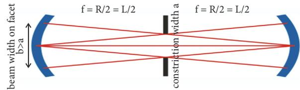
FIGURE 2: Principal sketch of the confocal resonator with constriction. The transverse beam width  $b$  on the facets is considerably larger than the opening width  $a$  of the low-pass spatial frequency filter in the middle plane.
