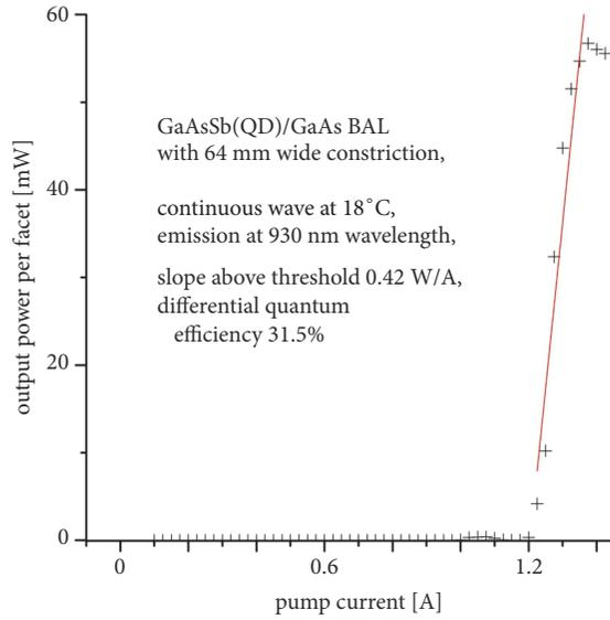
FIGURE 3: Laser characteristics of a confocal BAL with 64  $\mu\text{m}$  wide constriction just to show that the lasers are of very good quality. The laser threshold is at 1.2 A, and the output power per facet shows values around 60 mW for a pump current of about 16% above threshold.
