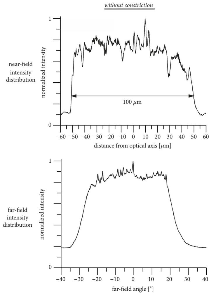
FIGURE 4: Near- and far-field intensity distributions for the confocal BAL without constriction, for comparison. The laser has been operated around 90 K in continuous-wave emission.
