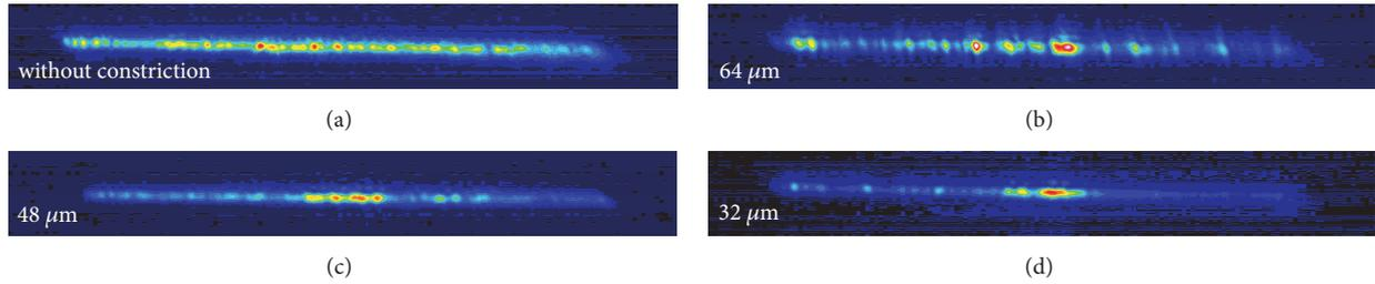
FIGURE 5: False-color plots of the near-field transverse intensity distributions for confocal BALs of the same batch with different widths of the constriction in the middle plane (i.e., no constriction, 64, 48, and 32  $\mu\text{m}$  wide, respectively). In all cases, the pump current has been around 16% above laser threshold and the lasers have been operated around 90 K in continuous-wave emission.
