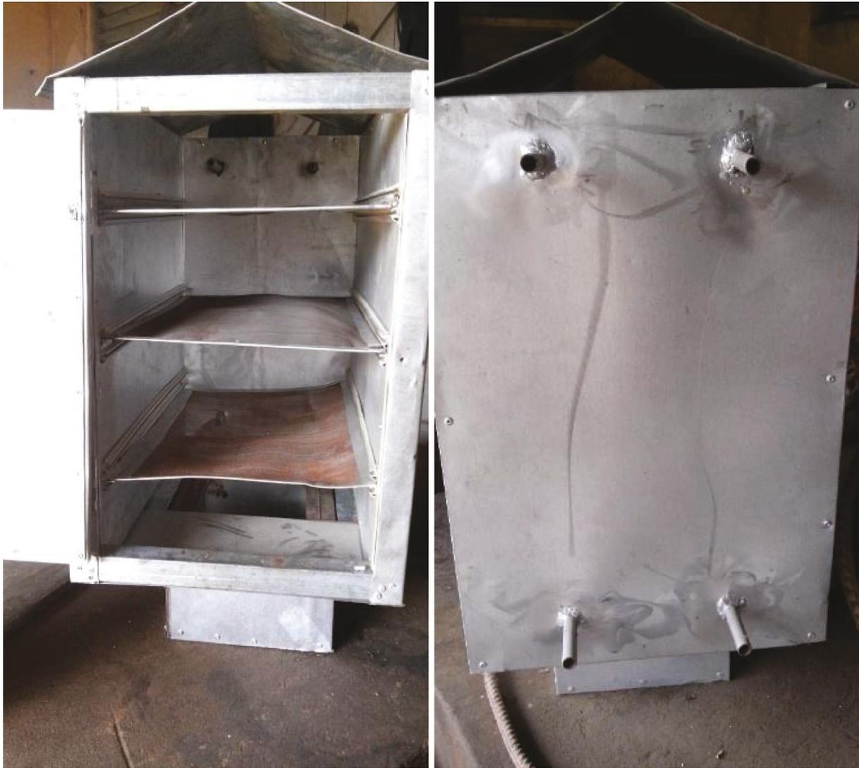
FIGURE 3: Front and rear views of manufactured smoke filter unit.
