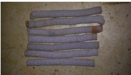
FIGURE 4: Polyurethane foam materials (mini-PUF) are used for passive sampling.
