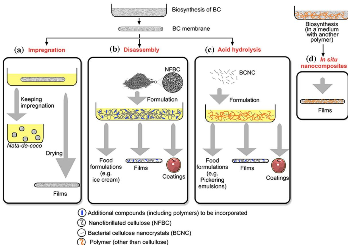
**Fig. 4** Techniques for mixing bacterial cellulose with other components for use in food packaging, **A** Impregnation; **B** Disassembly; **C** Acid hydrolysis and **D** In situ nanocomposites. Adapted from [130], reproduced with the permission from Elsevier
