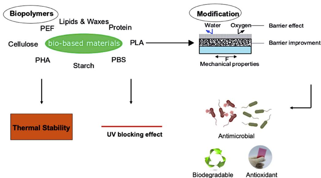
**Fig. 3** Biodegradable nanocomposite film and its properties (PHA Polyhydroxyalkanoate, PBS Polybutylene succinate, PEF Polyethylene furanoate, PLA Polylactic acid). Adapted from [20, 85], reproduced with permission from Springer and MDPI, respectively
