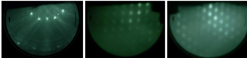
Figure 3. The left hand image shows a RHEED pattern from a (001) LAO substrate, [110] azimuth. Kikuchi streaks are visible, and diffraction maxima on arcs where the 2D reciprocal lattice rods intersect the Ewald sphere, indicating a smooth surface. The right hand images are from a 1900 Å \text{UO}_2 film grown on LAO. The surface is rougher and 3D spot patterns are observed, formed by transmission through 3D islands. The [100] and [110] \text{UO}_2 azimuths are shown, respectively. RHEED images have been adapted from Ref. [72]
