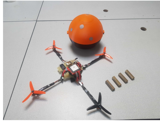
Figure 1: Quadrotor with additional masses and custom spherical body.
