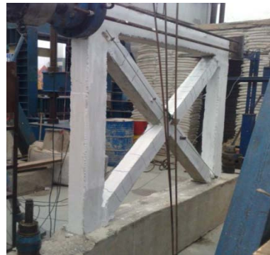
Figure 4. Mode of failure of F2
