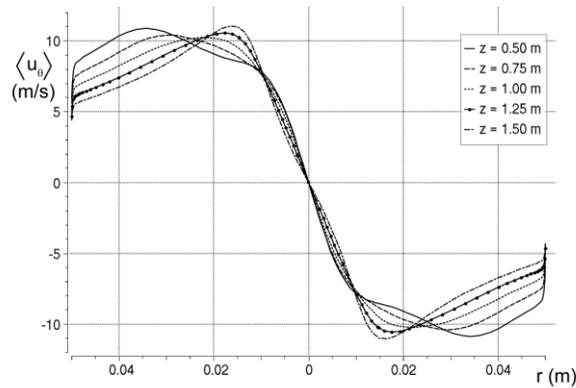
Fig.3. Tangential velocity profile along the axial direction (Najafi et al., 2011).
