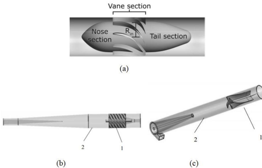
Fig.6. Structure of the internal swirl element(ISE) (a)Traditional separator, b) Spiral shape, c) Blade type. (Shi and Xu, 2015)
