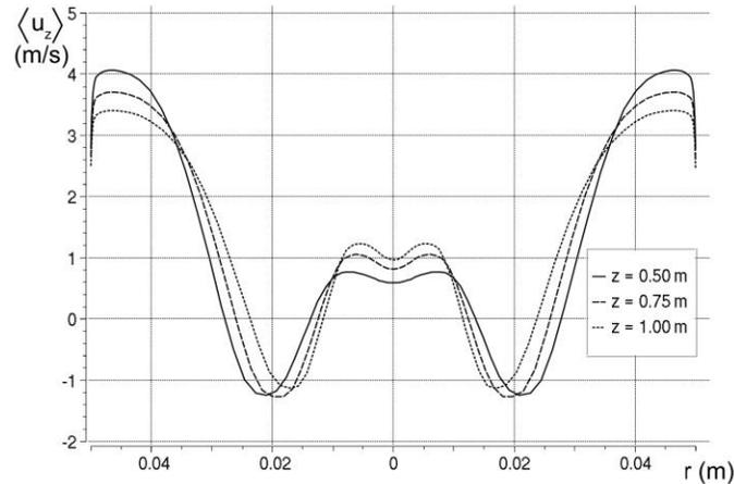
Fig.4. Axial velocity distribution at three axial sections
