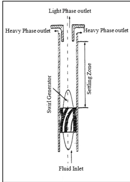
Fig. 2. Conventional type of the hydrocyclone (Dirkzwager, 1996).
