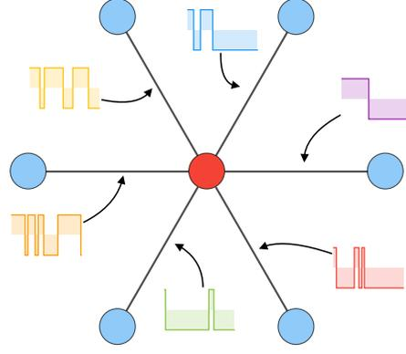
**Fig. 1.** Pictorial representation of the model described in Section 2: the links between the nodes of a graph (in this work, we focus on the star graph) are affected by independent sources of RTN, all characterized by the same switching rate  $\mu$  and noise strength  $\nu$ . The red node corresponds to the marked node in the Hamiltonian,  $|w\rangle$ .
