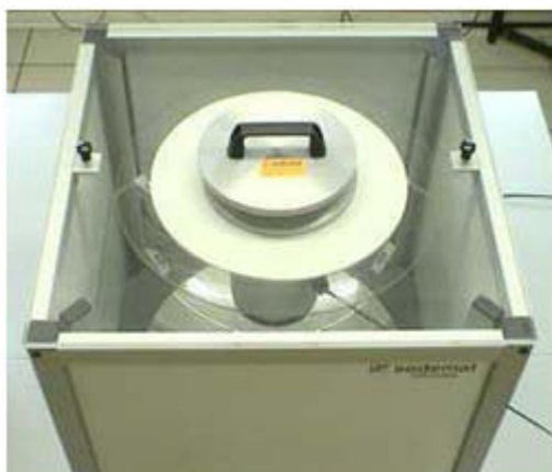
Figure 2. The Cusick drapemeter
