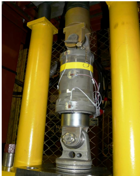
Fig. 8. The modified shock absorber on a stand during fatigue testing
