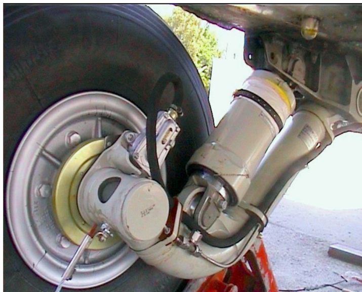
Fig. 1. The new main landing gear of PZL M28 aircraft
