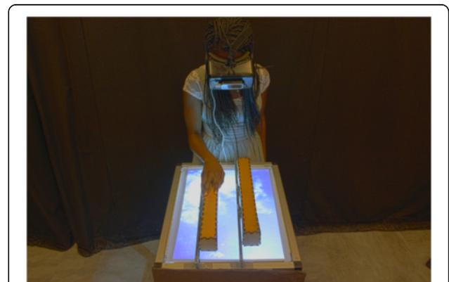
**Fig. 6** The TASC system establishes embodiment through a combination of virtual reality with head and hand tracking and physical feedback provided by the blocks, which can be grasped and moved
