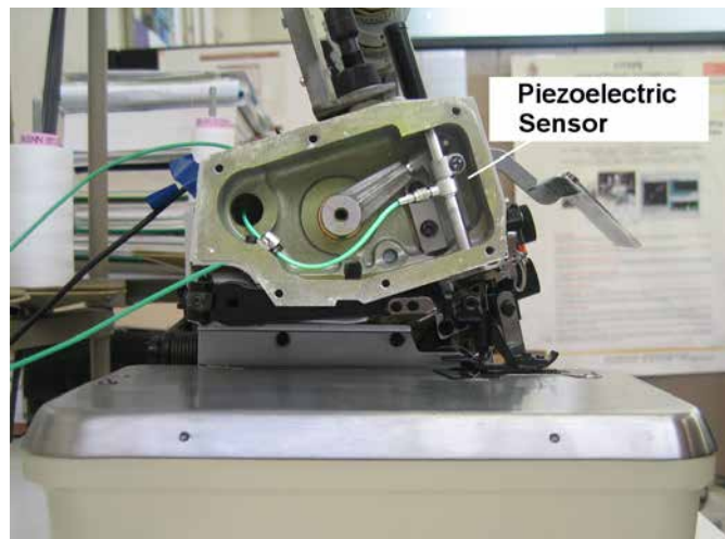
Figure 2. Setup of the piezoelectric sensor in the machine’s needle bar.
