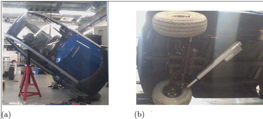
**Figure 1** Vehicle mechanical modification. (a) Tilting the vehicle using two axle stands, to enable access to the underside. (Note also lidar mounted to roof.) (b) Underside with linear actuator added for steering.
