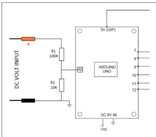
**Figure 6** Potential divider linked to the battery.
