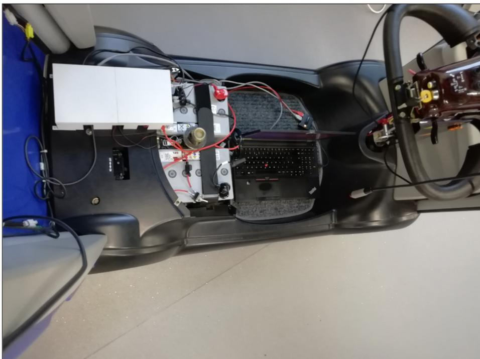
**Figure 4** PCB enclosure mounted on the vehicle (top left, white box).
