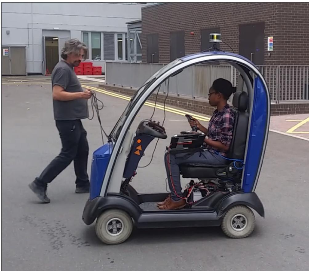
Figure 15 OpenPodcar test drive in remote control mode.
